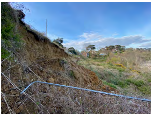
Photo 12. 3rd April 2020. Further continued slow translational failure and scarp development.
